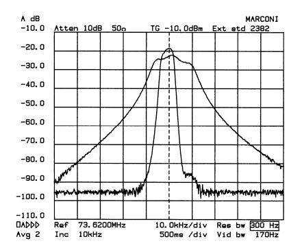
The result of the bandwidth improvement shown above is the reduction of close in intermodulation from multiple signals. The IMD dynamic range will be improved up to 10 dB for some tone spacings. The main receiver audio response will be reduced about 100 Hz in the SSB mode. Operating the noise blanker will not result is as much degradation of the dynamic range.
