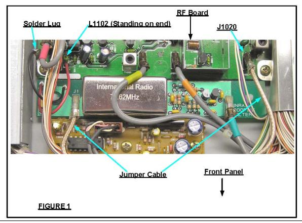
**Note:** If you remove the red coded coaxial cable in order to access the point of soldering the power wire, be sure to reconnect it back to J1008. If you reattach it to J1009, the radio will not transmit.
